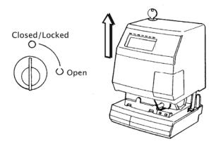
Figure 2-2. Auto-Sync Time Clock Cover Removal.
